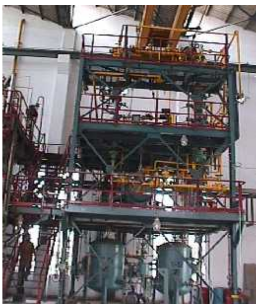
Fig 7.5: TBR Pilot plant Phase-II (6 & 12 inch column)
